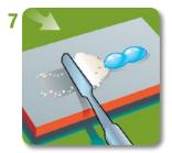
Add powder to liquid in one portion and mix. When properly mixed, material should stretch 1/2" from pad or slab.
